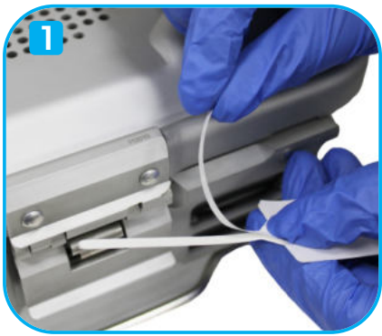
1 Unglue the tail section on the self-adhesive label.
